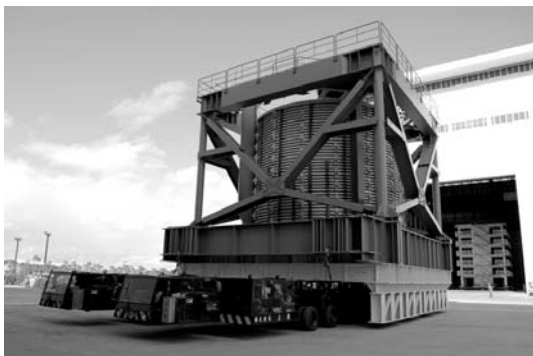
写真2.10 試験体の震動台への運搬 Photo 2.10 Specimen carried to the shaking table.
