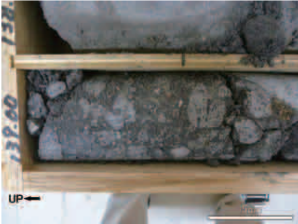
写真 19 深度 139.1 m, 凝灰角礫岩(火砕流堆積物) Photo 19 Scoriaceous tuff breccia (pyroclastic flow deposit): 139.1 m deep.
