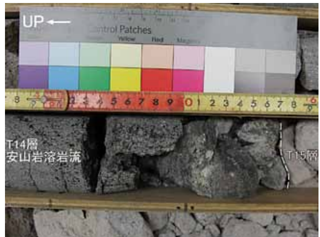
写真15 深度103.5 m, 安山岩質溶岩流の基底部 Photo 15 Basal fragmented part of andesitic lava flow: 103.5 m deep.
