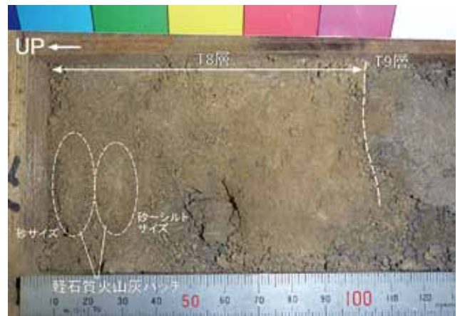
写真 9 深度 72.0 m, パッチ状の黄白色火山灰層を含む風化火山灰質土壌層 Photo 9 Weathered tephra-derived soil layer include patchy clumps of yellow white volcanic ash in 72.0 m deep.
