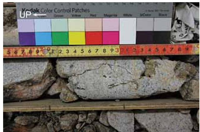
写真17 深度192.3 m, 岩塊表面や割れ目に沿って変質している凝灰角礫岩(火砕流堆積物) Photo 17 Altered tuff breccia (pyroclastic flow deposit): 192.3 m deep. Alteration has undergone along cracks and surface of blocks.
