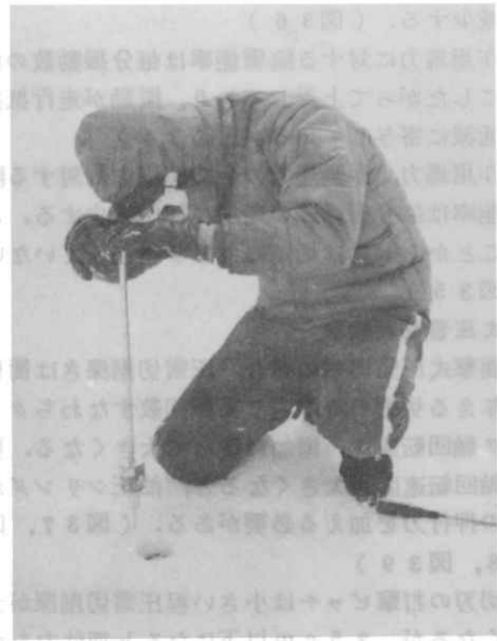
写真10 木下式硬度試験 Photo 10. Hardness test of compressed snow (Dr. Kinoshita's type).
