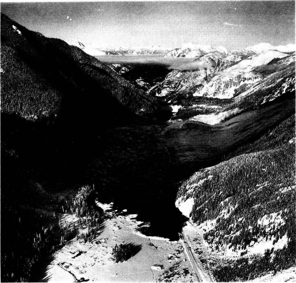
Fig. 5 Deposit of the 1965 Hope Landslide in British Columbia, Canada. The dark area in the forefront is the "splash" of liquefied valley deposits displaced by the rock avalanche. (B. C. Government Airphoto BC (0) 447).
