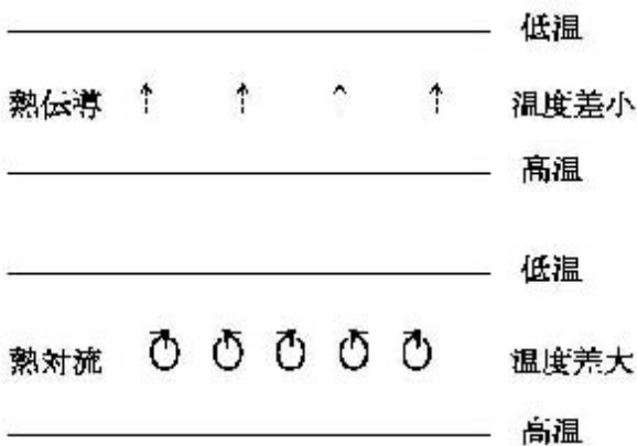
図3 非平衡系の発達の具体例 (熱伝導と熱対流) Fig. 3 Example of development of non-equilibrium system (heat conduction and heat convection).
