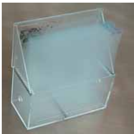
図5 ICソケットを収納ケース内側に取り付けた例 Fig. 5 A model which IC sockets are attached inside the container.
