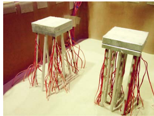
写真 2 遠心振動実験の斜杭模型(左)と直杭模型(右) Photo 2 Model of batter-pile (left side) and vertical-pile (right side).
