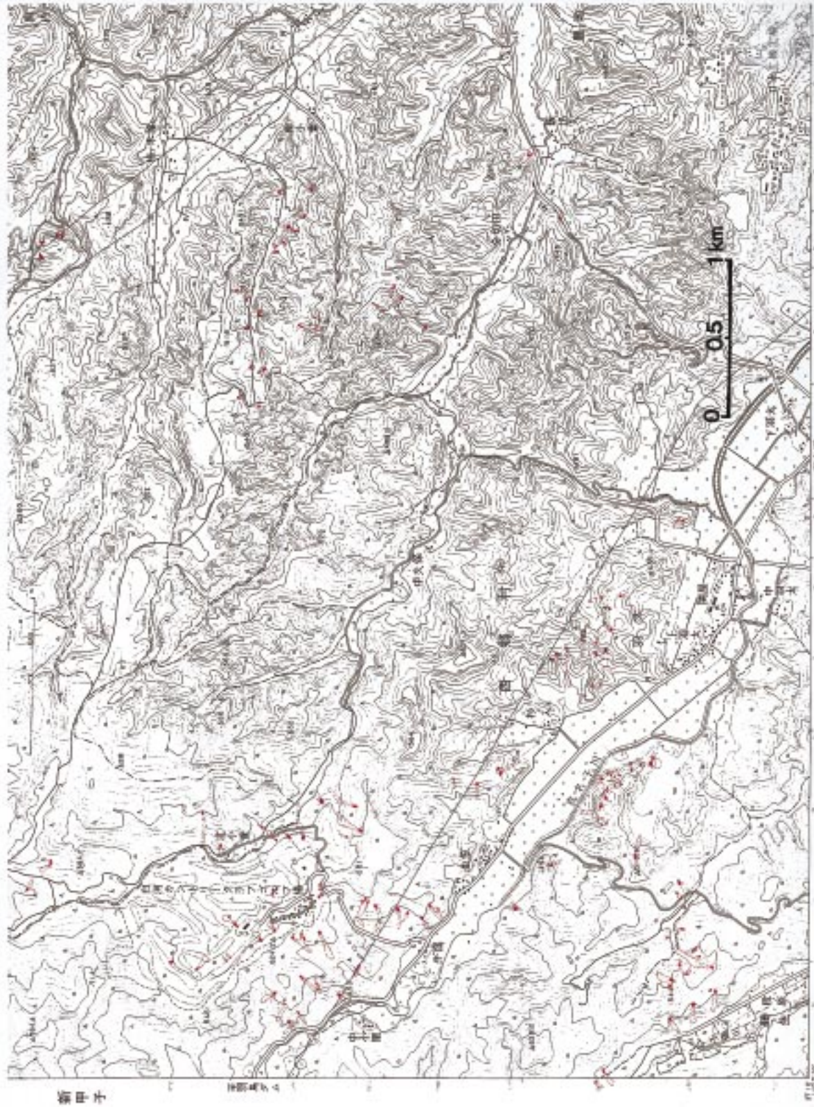
図12 西郷村羽太地区崩壊分布図 Fig.12 Landslide distribution in the Habuto district.
