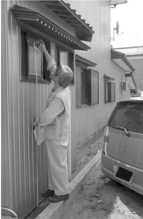
写真2 浸水深の計測状況 Photo 2 Measurement of the flood level.
