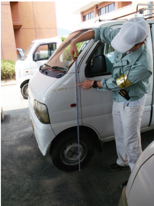
口絵6 堪野川流域での洪水痕跡調査 Fig. 6 Investigation of water level at the inundation along Fushino River.
