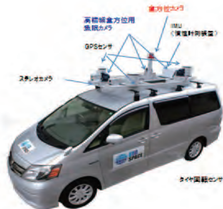
図28 360度全周撮影用カメラを搭載した車 Fig. 28 Car loaded with a special video camera for photographing 360° panoramic view.
