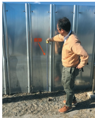
写真4 工事現場(M12)のフェンスに残される浸水痕跡 Photo 4 Water line from flood waters visible on the fence at investigation location M1.
